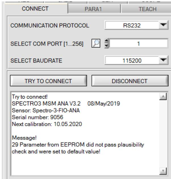
In the status window of the CONNECT tab, **Next calibration** indicates when the sensor has to be sent in for calibration.
