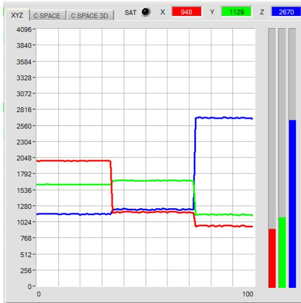
The newly added LED **SAT** indicates if one of the channels is in saturation. In this case, it lights up red.
